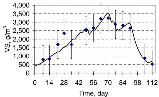
**Figure 3.** Biofilm growth and decay (VS, g/m<sup>3</sup>) vs. time: Data, diamonds; Monod model, solid line. Error bars are control blank mean standard error.
