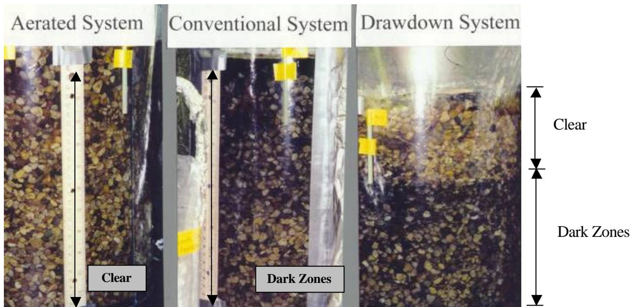
Figure 2 – Media photograph of aerated, conventional, and drawdown reactors. The media in the aerated reactors had little to no film or buildup along the length of the reactor. The media in the conventional reactors had a black zone along the length of the reactors. The drawdown reactors had black zones below the drawdown zone.
