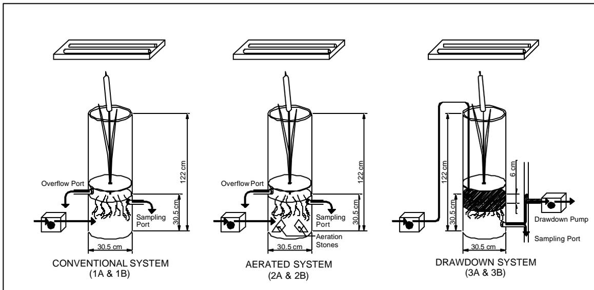
Figure 1 – Schematic of Conventional, Aerated, and Drawdown Systems
