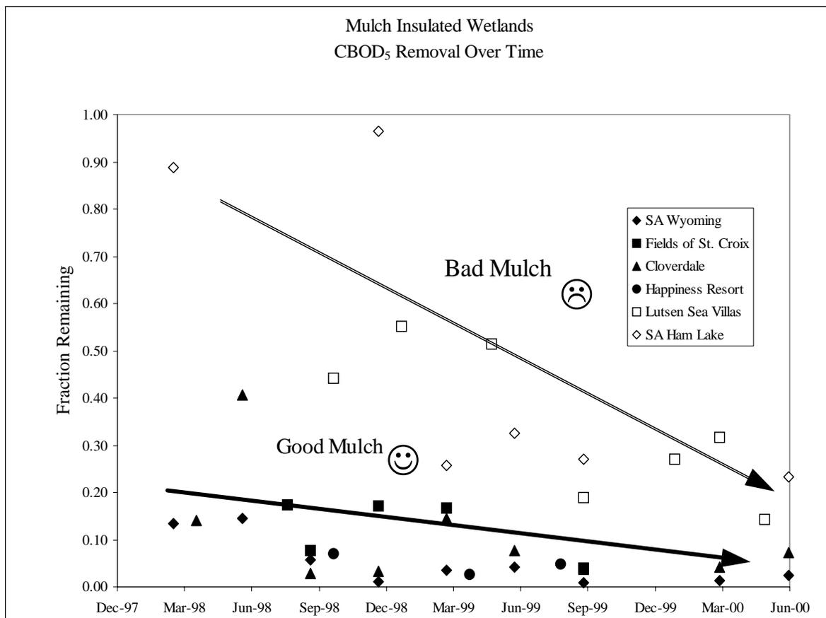
Figure 3: Summary of long-term trends in CBOD<sub>5</sub> removal for six mulch-insulated subsurface flow wetland systems located in Minnesota. Systems represented by black data points were constructed with good mulch. Systems represented by white data points were constructed with bad mulch.
