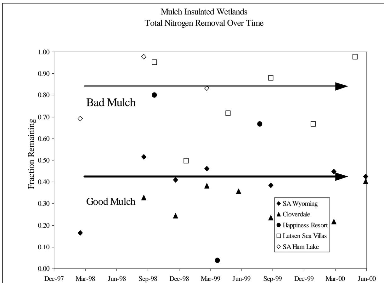
Figure 4: Summary of long-term trends in Total Nitrogen removal for five mulch-insulated subsurface flow wetland systems located in Minnesota. Systems represented by black data points were constructed with good mulch. Systems represented by white data points were constructed with bad mulch. None of the systems were aerated.
