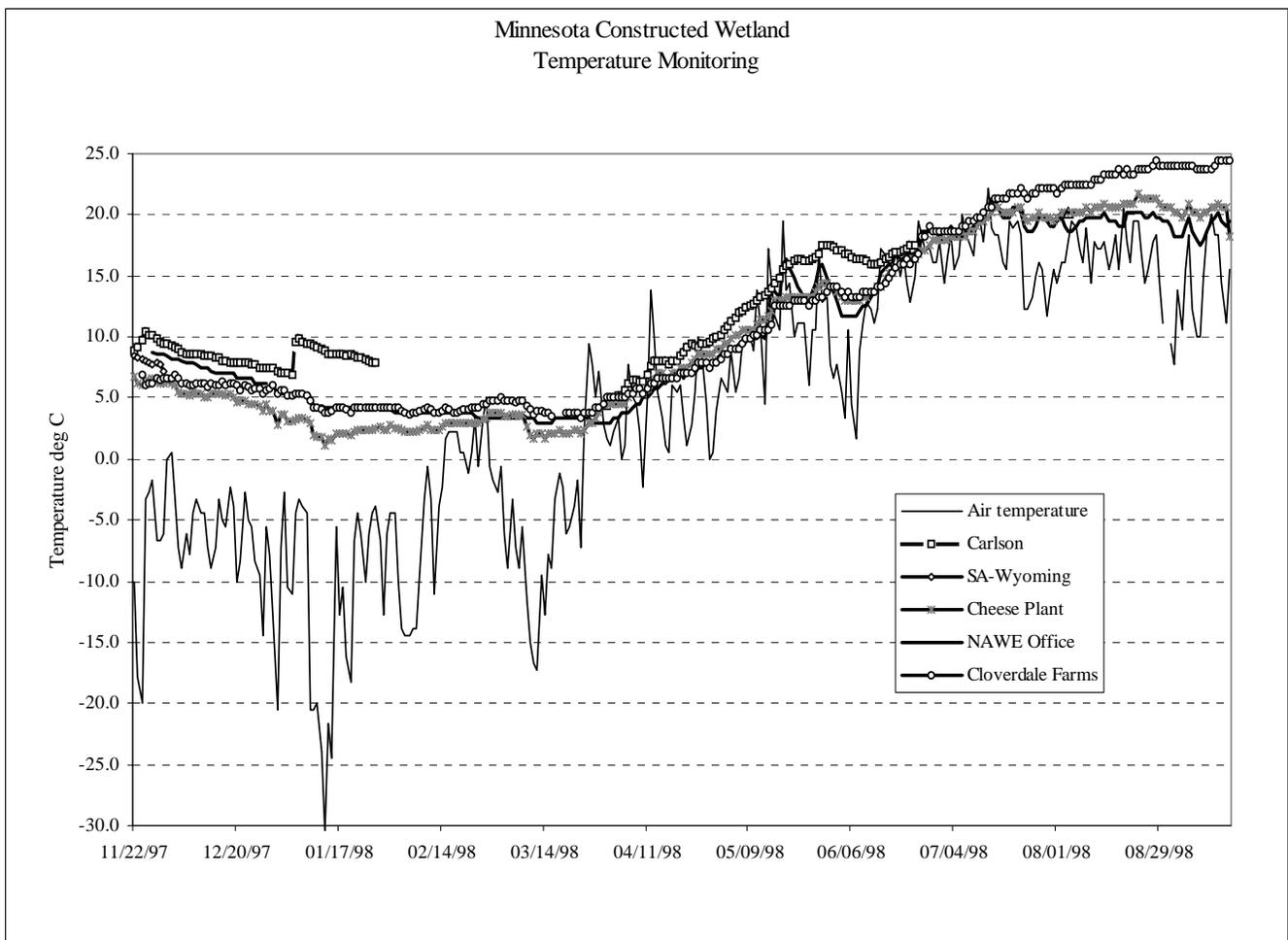
Figure 2: Effluent temperatures for five mulch-insulated subsurface flow wetlands located near Minneapolis, Minnesota. In one of the systems (Carlson) the hot tub was dumped to the septic tank, resulting in the temperature spike seen on the left hand side of the graph.
