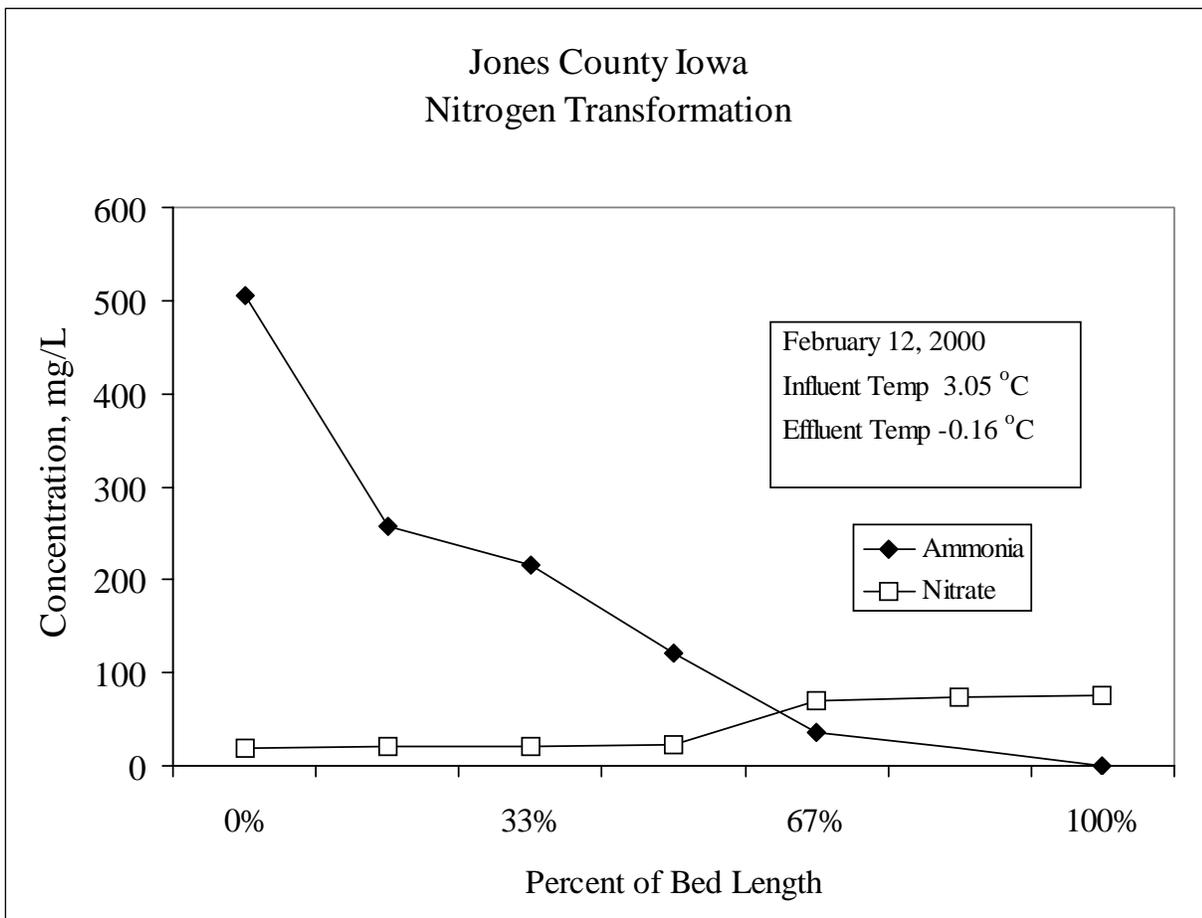
Figure 5: Ammonia and nitrate concentrations along the main flow path of the mulch-insulated subsurface flow wetland at the Jones County Landfill on February 12, 2000. This system was aerated to remove oxygen limitations to nitrification. Due to the high levels of total dissolved solids in the landfill leachate, the effluent temperature was depressed below 0 °C.
