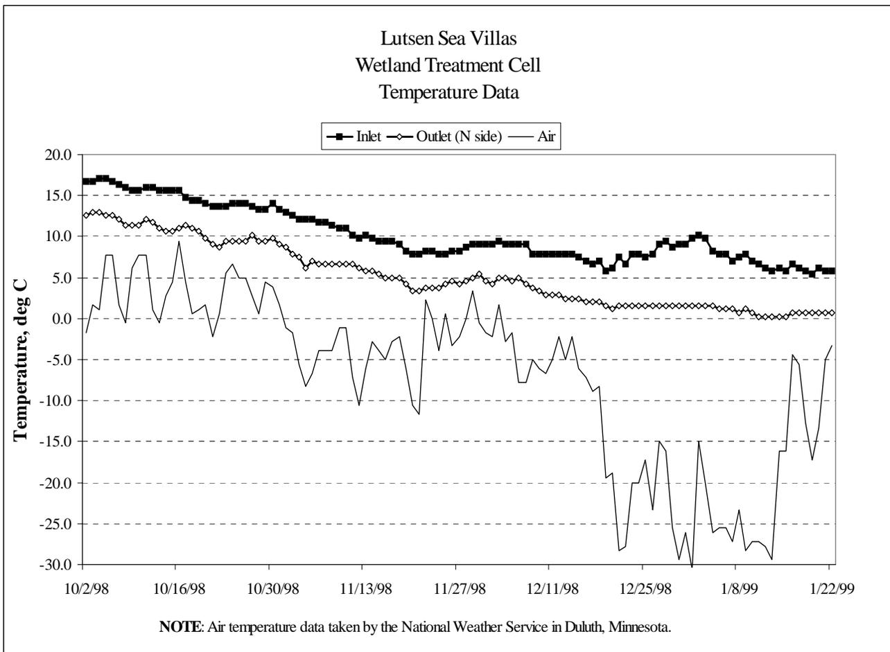
Figure 1. Temperature response of mulch-insulated subsurface flow wetland at Lutsen Sea Villas during extreme freezing event in December 1998 and January 1999.
