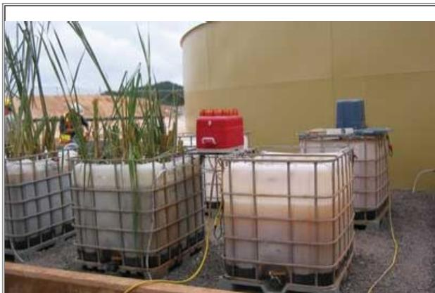
Pilot unit used to evaluate treatment of mine tailings water by a wetland system.
